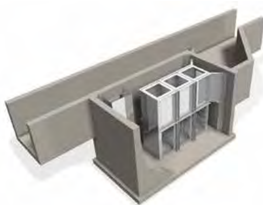
Typical Off-Line Ecosol GPT configuration
