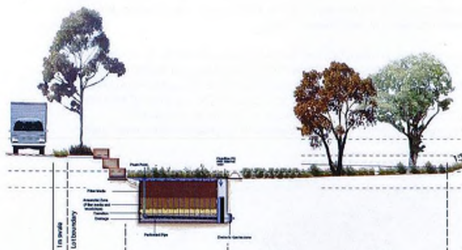
Figure 7.10 Section through detention basin showing a saturated zone bioretention and bund (small) separating it from the larger basin footprint
