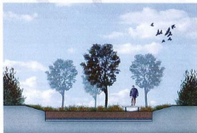
Figure 7.12 Section illustrating path within the detention basin
