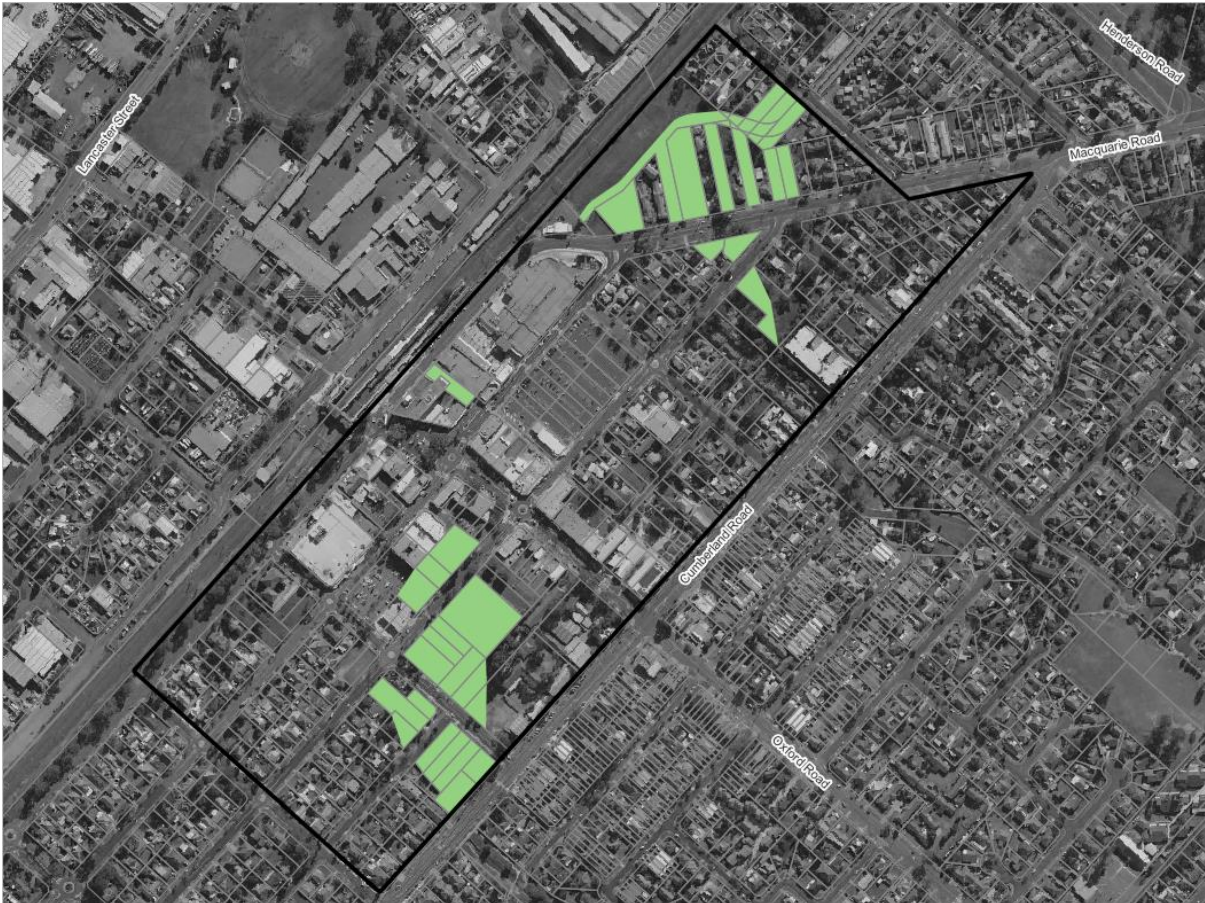
Figure 11 Lots exposed to H5 or H6 hazard at the peak of the PMF (Green)
