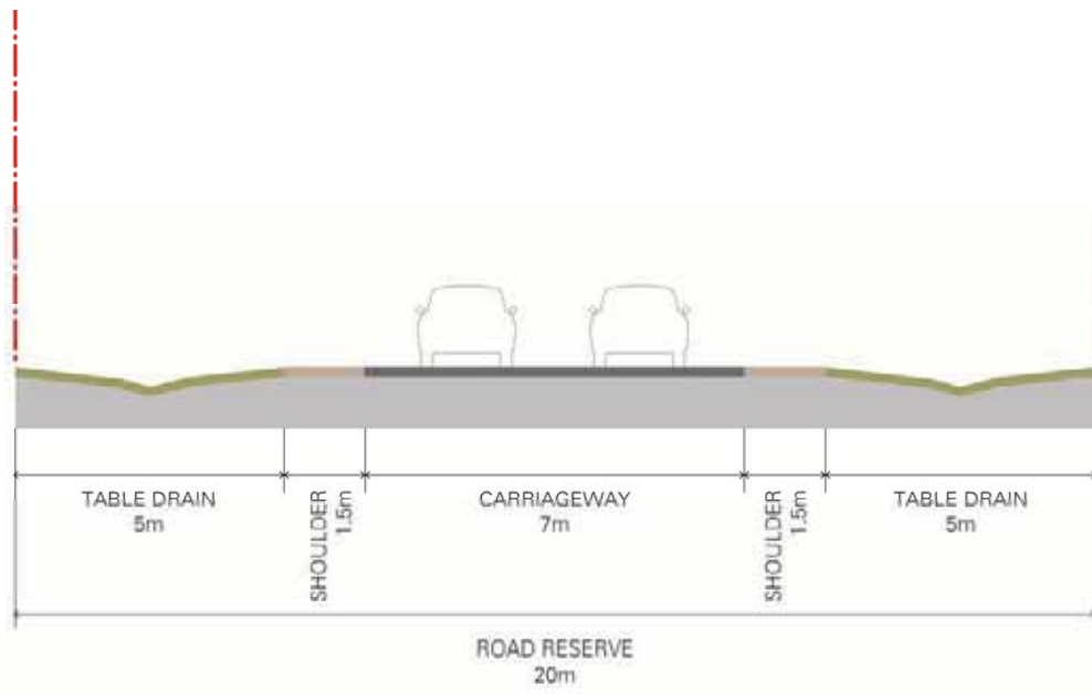
Figure 16 - Typical Rural Road section
