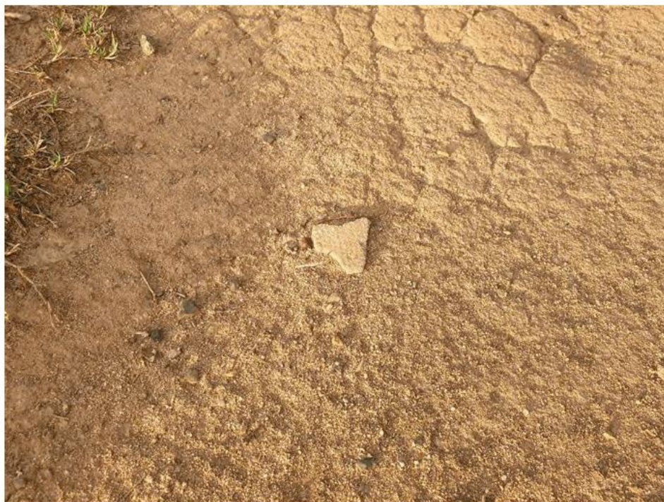
Plate 3 – Fragment of ACM (MS01) observed on the surface of the Site adjacent BH02
