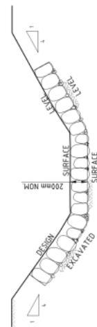
TYPICAL RIPRAP/SCOUR PROTECTION APRON SECTION
