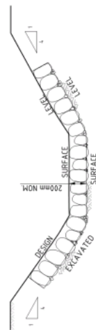
TYPICAL RIPRAP/SCOUR PROTECTION APRON SECTION
