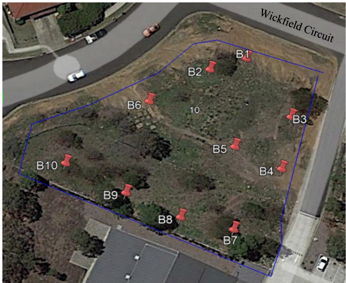
Figure 2.2: DSI Version 2 Sampling locations. BH1 turned into a monitoring well 4.5m depth.
