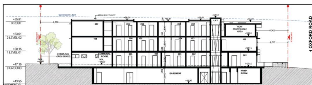
Figure 2: Extract from Section AA showing the minor non-compliance of the proposed development with the 9m Height of Building Development Standard.
