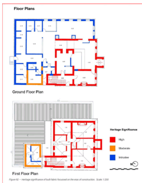
Figure 36 - Significance grading diagrams. It should be noted that all fabric of High significance will be retained, with only minor changes to the structure graded as being of Moderate significance at the rear of the former bank. Sourced from the CMP.
