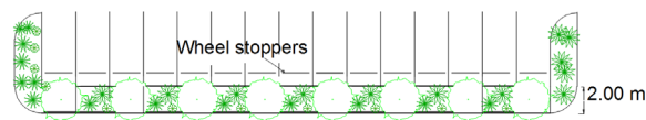
Figure 5.5.1 - An illustration of the need to use wheel stoppers to protect landscaping and the need to landscape all parking edges and between parking bays.
