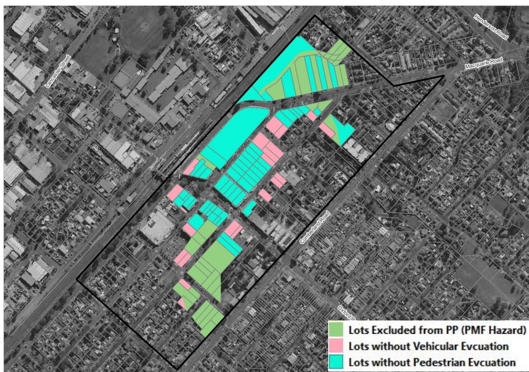
Figure 12 Lots exposed to H5 or H6 hazard at the peak of the PMF or with evacuation difficulties in the 1% AEP Flood
