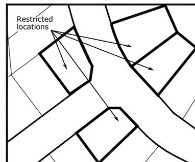
Figure 7.3.1 - An illustration of lots that may present potential vehicular/pedestrian safety hazard.
