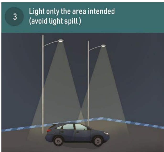
Figure 2: Use of shielding to minimise upward light spill from streetlighting
