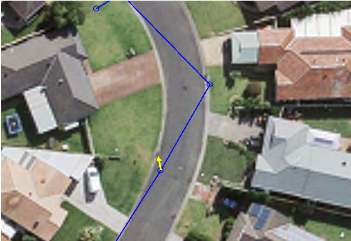
Plate 2 Example of incorrect spatial positioning of stormwater pit
