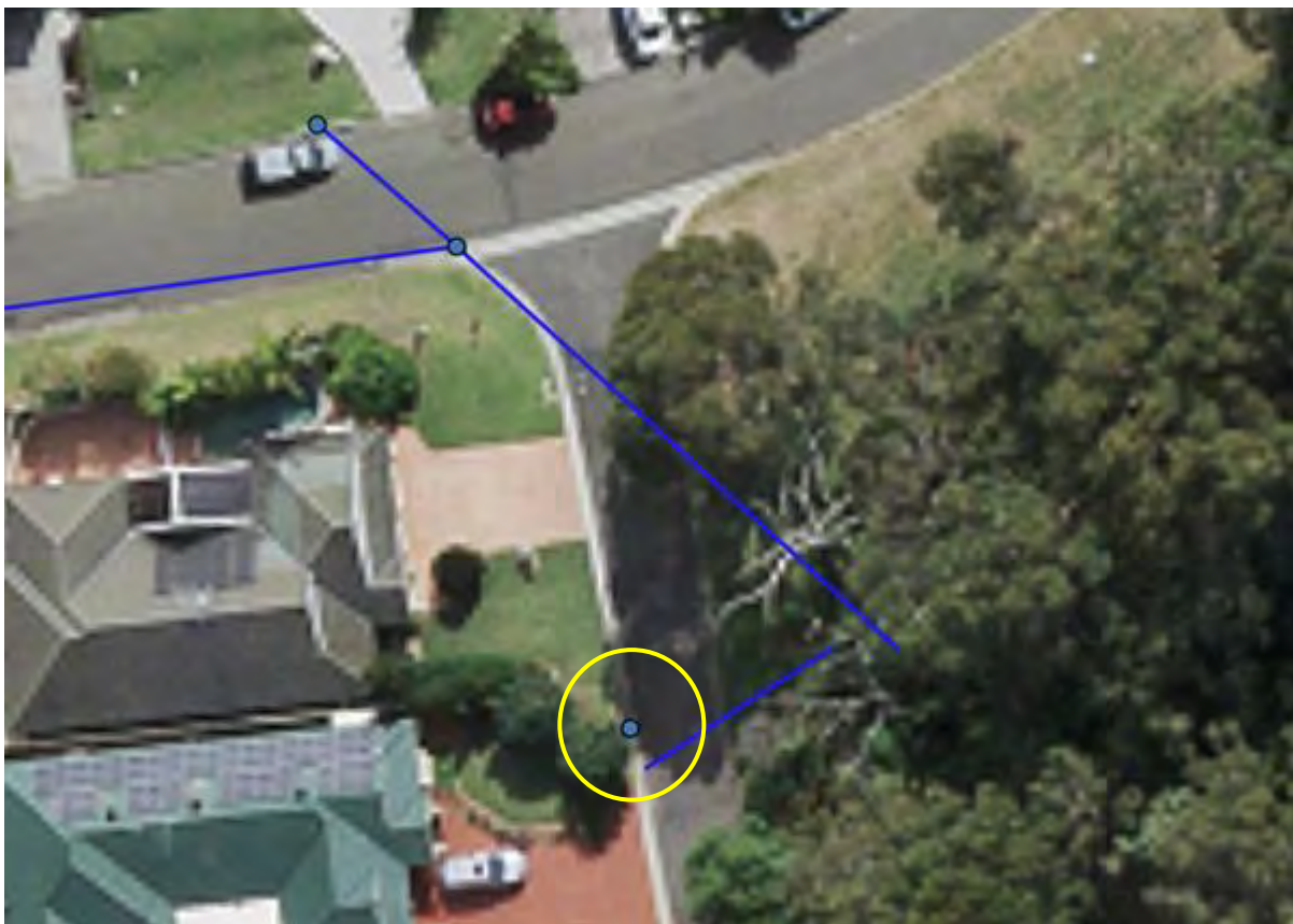
Plate 3 Example of disconnected stormwater pit and pipe
