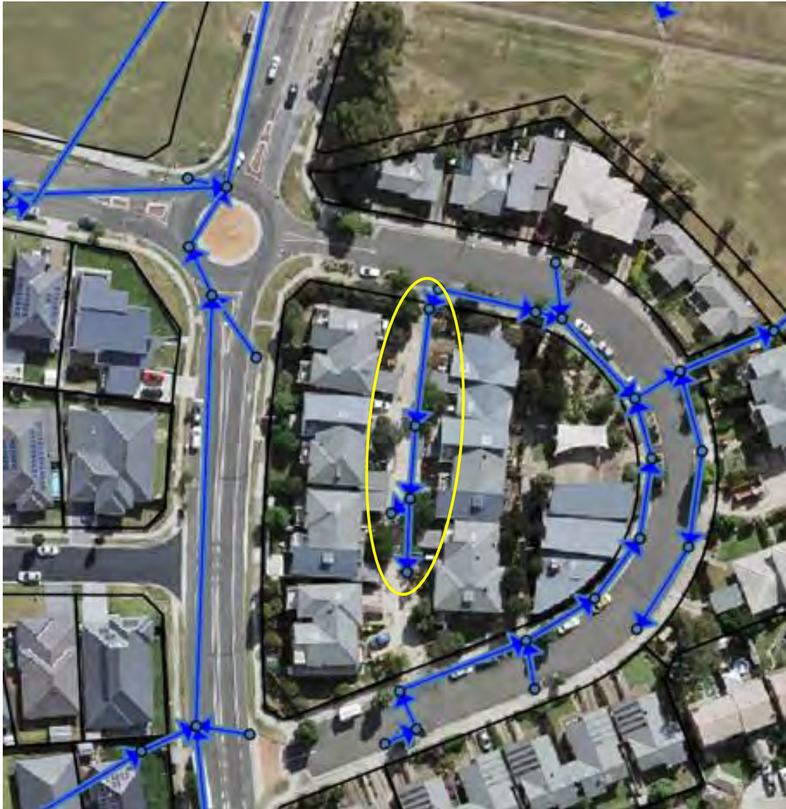
Plate 4 Example of incorrect pipe direction
