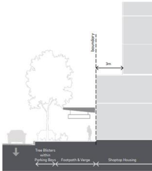
Figure 7.5 – Main Street Section – Non-Residential Interface
