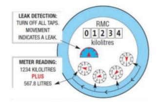
Kilolitres are shown by the black digital display and litres by the dials. The dials are read from right to left. When a pointer rests between two numbers use the lower number. The current reading on this meter is the same as the one on the previous page: 1,234 kilolitres and 567.8 litres or 1,234.5678 kilolitres.
