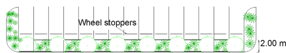
Figure 6.4.4.1 - An illustration of the need to use wheel stoppers to protect landscaping and the need to landscape all parking edges and between parking bays.
