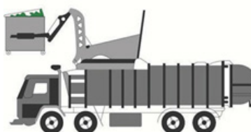
Figure 2.15.4 - Example of Front-lift waste collection vehicle
