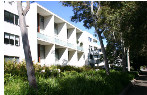
Figure 5.5.2 The provision of 20% of the site for deep soil planting can aid the aesthetics of the development.
